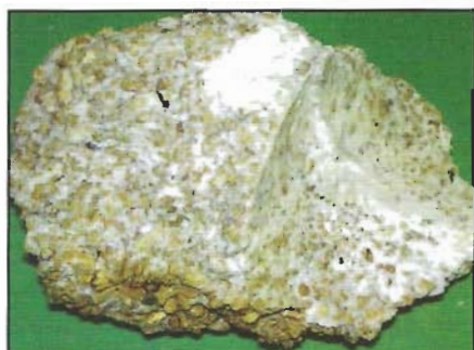
A typical sample of ground surrounding a leak point in a pipeline after application of Sanipor
